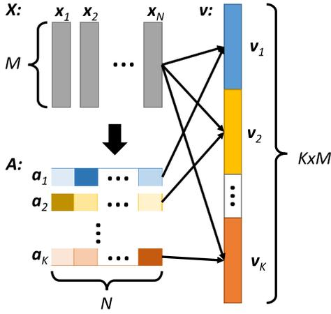
Fig. 4. Illustration of the proposed sparse self-attention module. The attention vectors  $\mathbf{a}_1, \dots, \mathbf{a}_K$  are generated by different non-linear functions with the local spatio-temporal features  $\mathbf{x}_1, \dots, \mathbf{x}_N$  as input. After  $K$  times weighted addition of the local spatio-temporal features by the attention vectors, we get  $\mathbf{v}_1, \dots, \mathbf{v}_K$  and concatenate them into a vector  $\mathbf{v}$  for the final motion representation.
